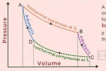
A Carnot heat engine is an engine that operates on the reversible Carnot cycle. The basic model for this engine was developed by Nicolas Léonard Sadi Carnot in 1824.
